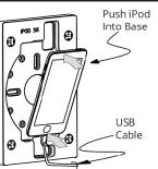
OPTIONAL: If a power solution is in place, connect the iPod's lightning cable now to confirm it's working.
