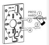
With the BASE piece positioned where vou'd like it to be installed, use vour choice of wall screw, and use it to mark the (4) anchor / mounting locations.
