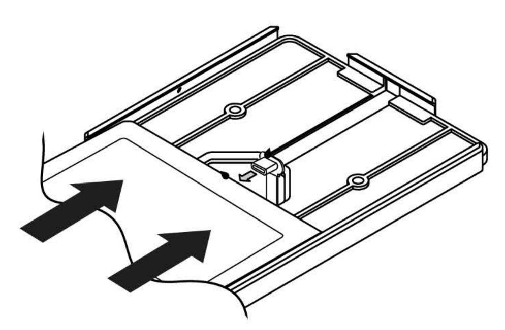
[B5] ... Carefully feed any cable slack into the empty space in the Mobile Part. Confirm the cable isn't pinched and doesn't have any sharp bends (this can cause cable damage).
