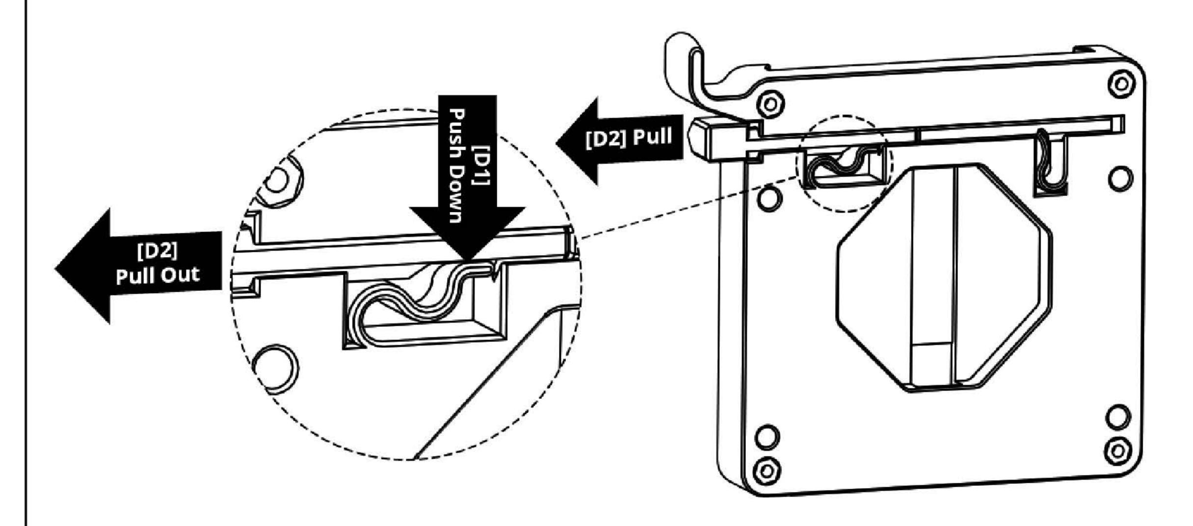
[D1] Facing the back of the Affixed Part, using your right hand, push down on the horizontal S-shaped spring.
