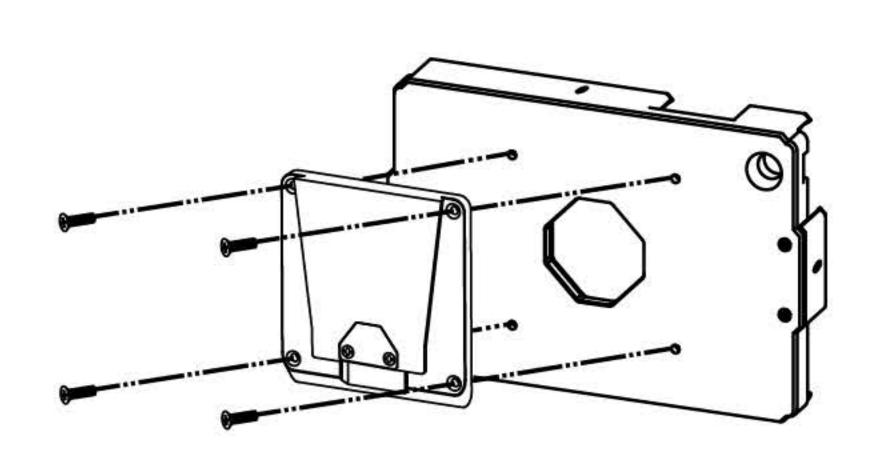
[B3] Carefully feed the preinstalled ribbon cable through the enclosure's back center hole.
