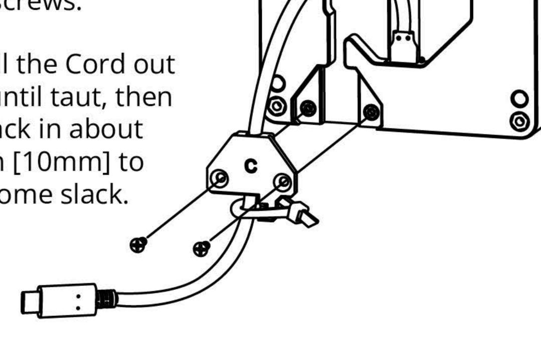
[G6] Zip-tie the cord in place to prevent cord from being pulled out or damaged.
