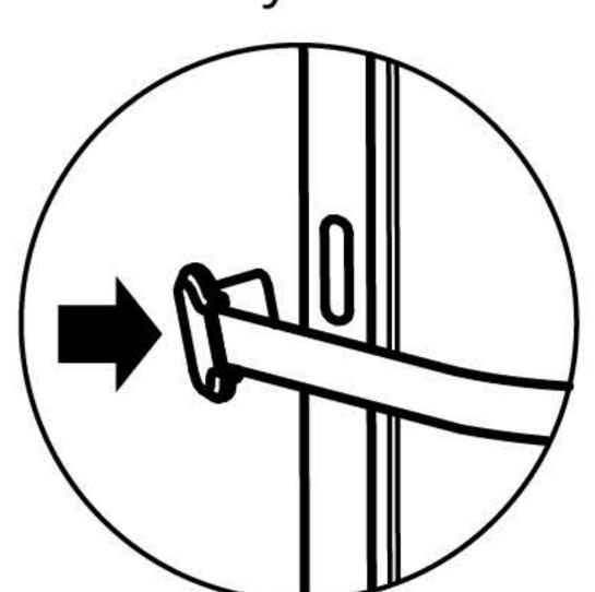
[C2] Carefully feed any cable slack into the empty space of the Mobile Part.
