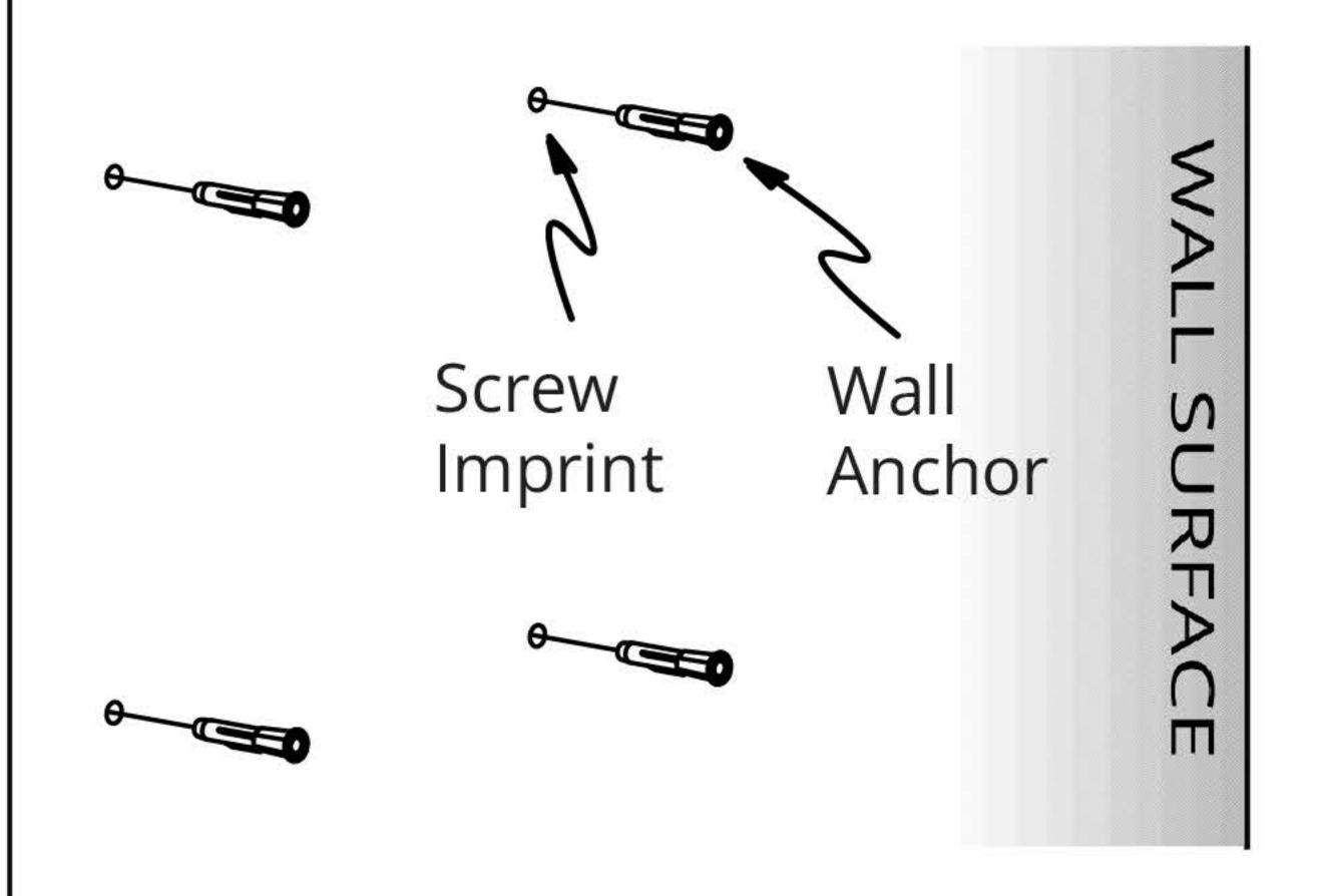
[I4] With the (4) anchor positions marked, install the (4) included wall anchors.
