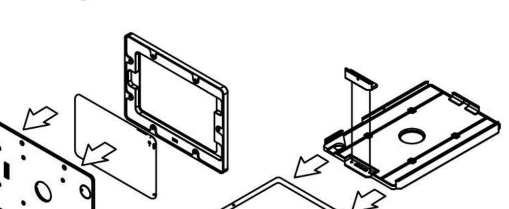
[B2] Using the (4) M4 x 10mm flat-head screws, assemble the Mobile Part onto the back of the VESA enclosure.
