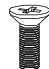
(Set D) M4x10 Phillips Countersink Head Screws (x2) [To secure Tilting Bracket together]
